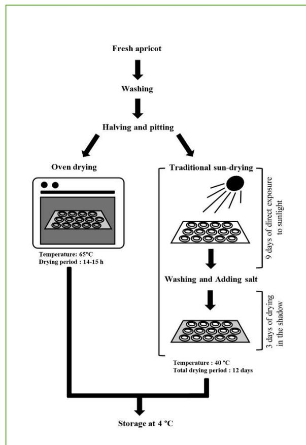
Figure 1: Simple schematization of the drying processes
